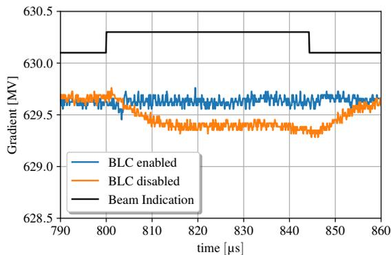
Figure 7: Cavity gradient with BLC enabled and disabled for beam with 50 bunches with 0.25 nC @ 1 MHz repetition rate.
