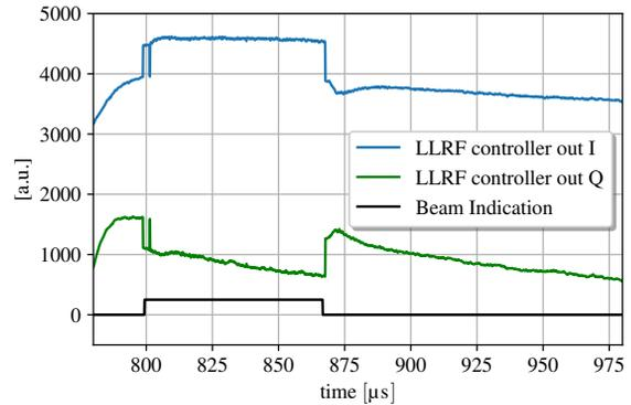
Figure 8: Controller output with the BLC enabled for beam with 300 bunches with 0.25 nC @ 4.5 MHz repetition rate.
