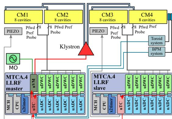
Figure 1: Simplified block diagram of the LLRF system installed at one RF station in XFEL.
