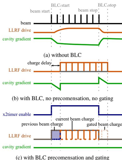
Figure 3: Beam loading compensation and cavity gradient.
