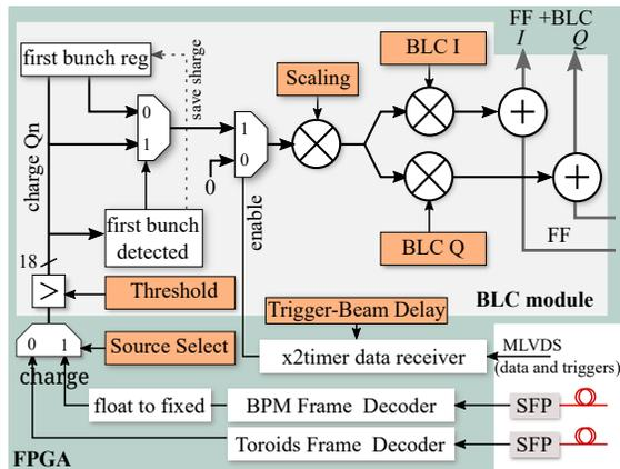
Figure 5: Block diagram of BLC module implementation.
