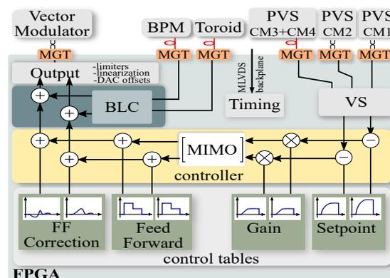
Figure 4: Block diagram of the uTC firmware including the most important components of the LLRF controller.
