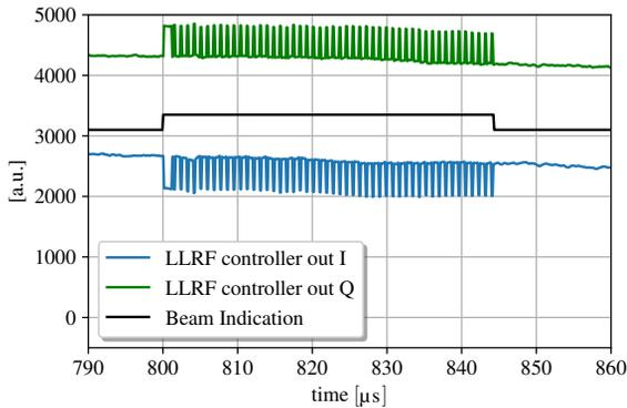
Figure 6: Controller output with the BLC enabled for beam with 50 bunches with 0.25 nC @ 1 MHz repetition rate.
