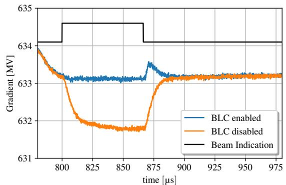
Figure 9: Cavity gradient with BLC enabled and disabled for beam with 300 bunches with 0.25 nC @ 4.5 MHz repetition rate.
