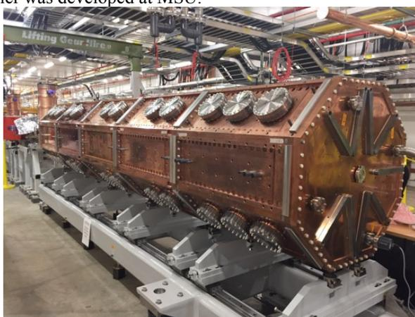
Figure 3: FRIB RFQ in the FRIB tunnel.
