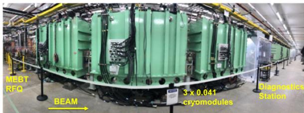
Figure 6: Three beta 0.041 cryomodules with the D-Station.
