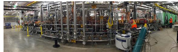
Figure 4: LEBT (left), RFQ (centre), MEBT (right), and 0.041 cryomodules (far right) in the FRIB tunnel.
