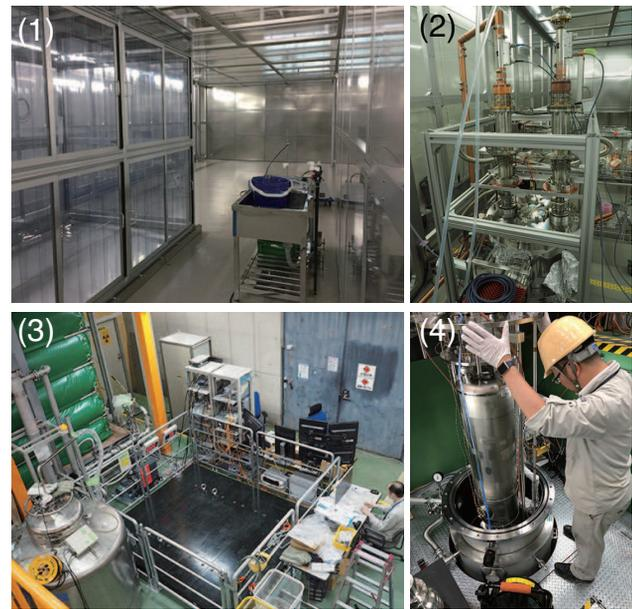
Figure 4: Photos of SRF infrastructure: (1) ISO Class 1 horizontal-flow clean room looking downstream, (2) Coupler test stand in clean room, (3) View of vertical test booth, and (4) Installation of bulk superconducting cavity into the test cryostat for vertical testing (VT).
