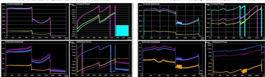
Output forward and reflection amplitudes and phases in case of using the phase modulation, RF station A6.L3 Gradient 760 MV
