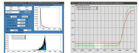
Partial discharges distribution for the time position and amplitude, A19.L3
