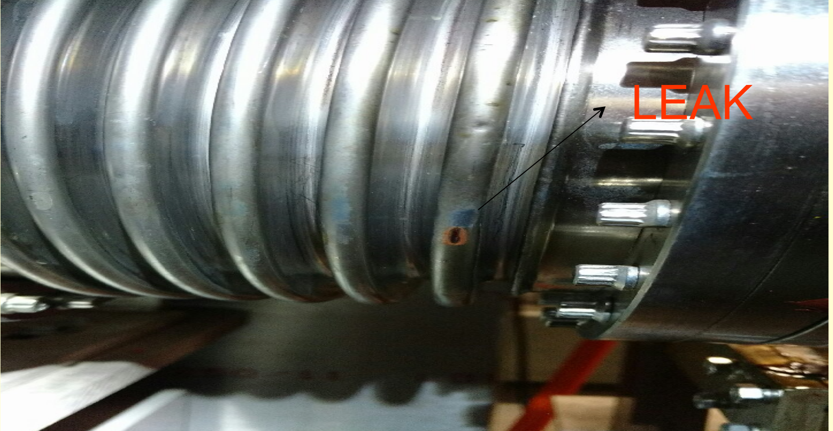
Figure 7: Hole in the bellow after the magnet chamber consistent with proton trajectory
