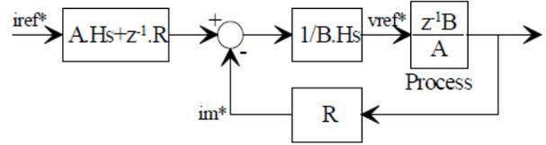
Figure 2: RST controller block diagram
