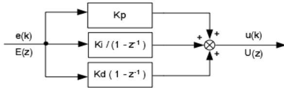
Figure 1: PID algorithm block diagram
