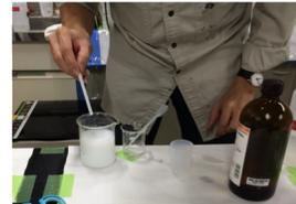
Recycle process was developed in RIKEN (Used target was dissolved in HF)
