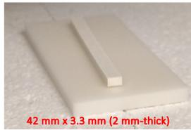
Sintered enriched target made in BNL
