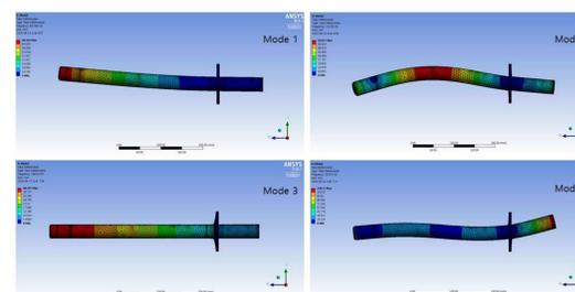
Figure 10. Vibrational modes of antenna
