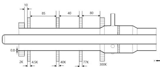
Figure 7. Scheme of a prototype power coupler for thermal analyses
