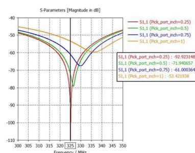
Figure 5. Effect of pick-up port diameter change
