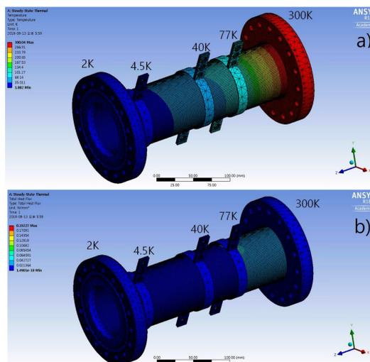
Figure 8. a) Temperature distribution and b) Heat flux result of static thermal load
