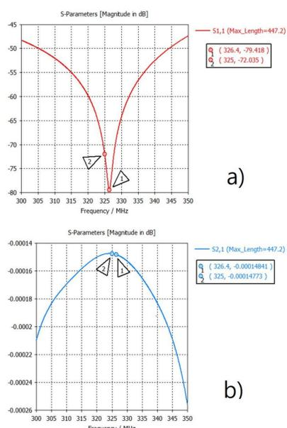
Figure 6. a) Reflected power ( $S_{11}$ ) b) Transmitted power ( $S_{21}$ ) of power coupler
