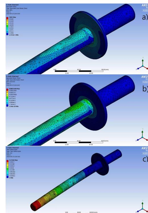
Figure 9. a) Stress, b) Strain, and c) Deformation of inner conductor and ceramic window
