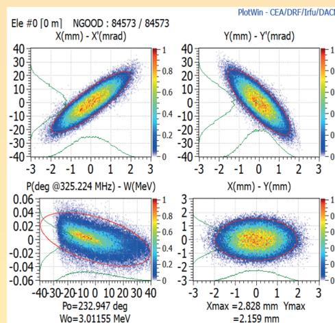
Figure 3: Phase-space plots and distribution projections (green curves) at the RFQ exit ( $10\text{ mm}$  behind the electrode ends) in the case of an entrance current of  $100\text{ mA}$ . The colors of the scatter plots refer to the normalized (macro) particle density (linear scales at the right frames of the plots). The red ellipses correspond to the  $95\%$  emittances.
