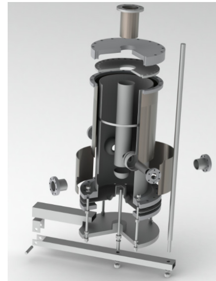
3D model for copper prototype manufacturing (RF and measurement loops are not visible) MEPHi (Russia)
