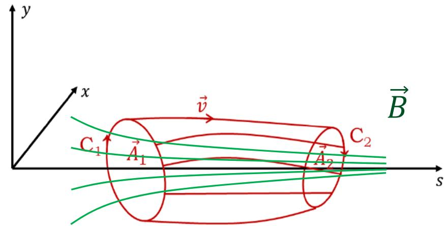
Theorem states preservation of axial canonical angular momentum in presence of axial B-field. "Canonical" means that the magnetic vector potential is included into the momenta (conjugated momenta)
