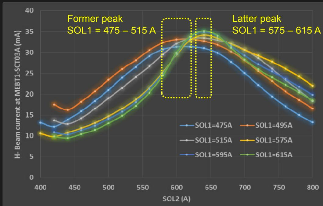
Dependence of H- beam current measured at MEBT-SCT to the SOL 1 & 2 current
