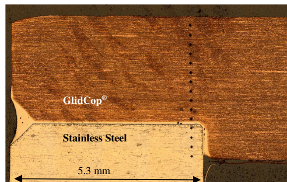
Figure 3: Stainless steel to GlidCop ® vacuum braze.
