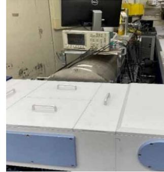
Figure 1: Far-IR 2m gas cell and Bruker<sup>©</sup> spectrometer.
