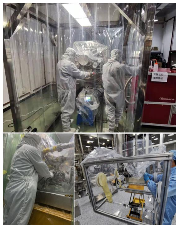
Figure 2: Moveable laminar flow booths for local particle-free assembly.
