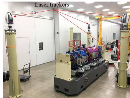
Figure 2: Laser tracking interferometer system.
