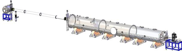
Figure 1: X-ray scattering experiment vacuum camera device.
