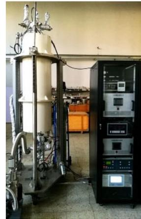
Figure 1: Prototype of NEG coating facility.
