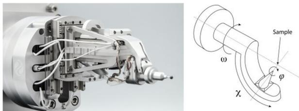
Figure 1: SmarGon with a representation of the rotations  $\omega$ :  $[-\infty, +\infty]$ ,  $\chi$ :  $[0, 90^\circ]$ ,  $\varphi$ :  $[-\infty, +\infty]$ .
