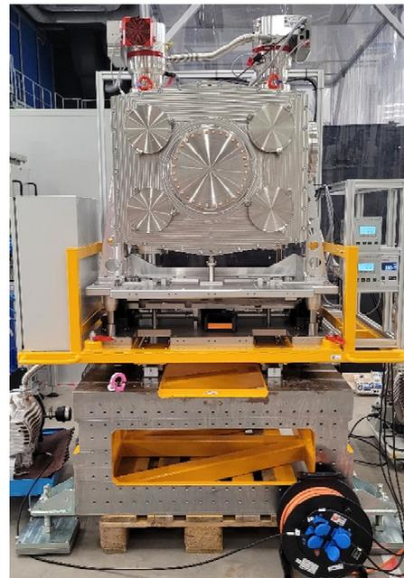
Figure 2: Assembled mechanics of the MDS on separate girder with air pads.
