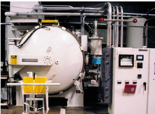
*A view of one of Fremont's high temperature vacuum furnaces shown with the cryogenic vacuum pump and Honewell controls and recorders.*
