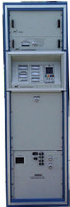
**20 KW, 402 mHz, RF Amplifier designed and built for LBL (SNS)**
