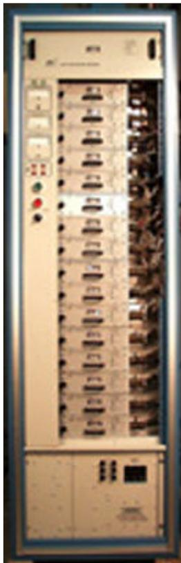
**8 KW, 211 mHz RF Amplifier designed and built for BNL (NSLS)**
