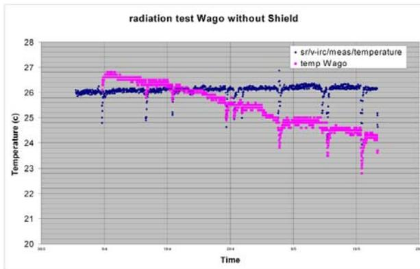
Figure 2: Temperature profile of an unshielded PLC.
