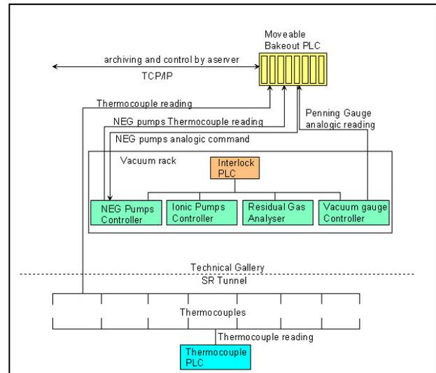
Figure 3: Layout of bake-out monitoring.
