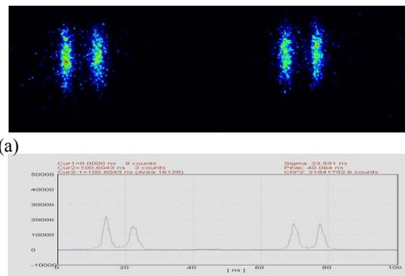
Figure 2: Image on the streak camera. The bunch profile (a) and its projection to horizontal axis (b) are shown.
