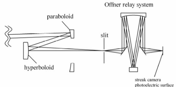
Figure 1: Reflected optical system of the streak camera.
