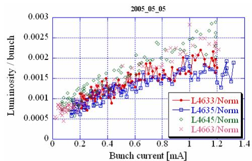
Figure 5: Bunch by bunch luminosity in HER condition d) in Table 1 and 2. The symbols are the same as in Figure 4.
