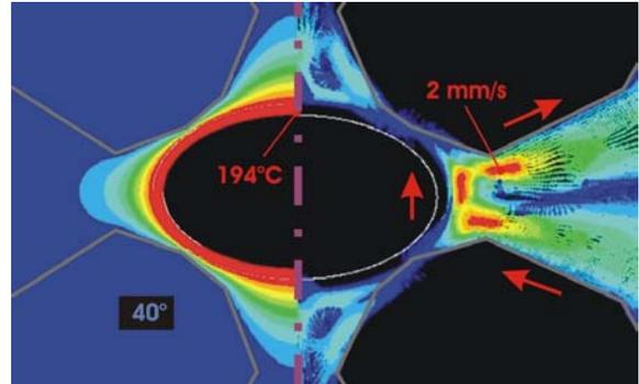
Figure 5: Temperature distribution (left) and velocity field of convection (right) at  $523 \text{ W/m}$  heater power.
