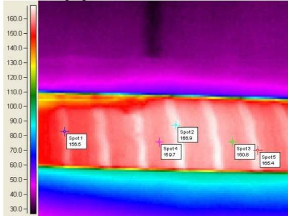
Figure 6: Thermography of heater (no reflective screen)
