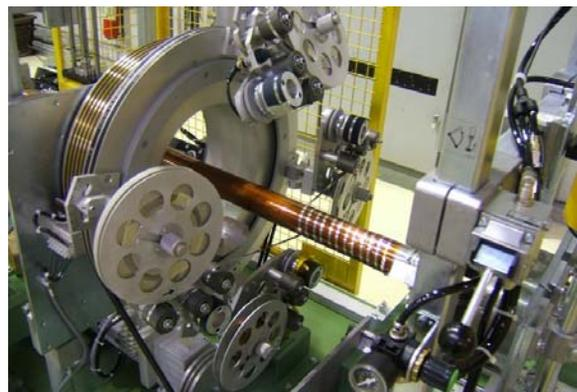
Figure 2: Simultaneous wrapping of two heater bands.
