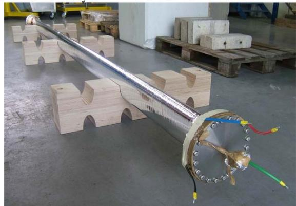
Figure 1: Finished MBXW chamber.
