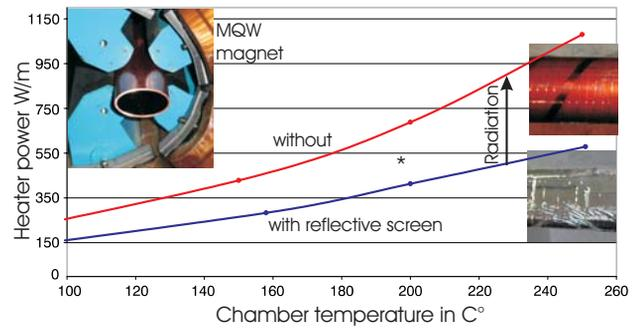
Figure 4: Bake-out test of MQW chamber.
