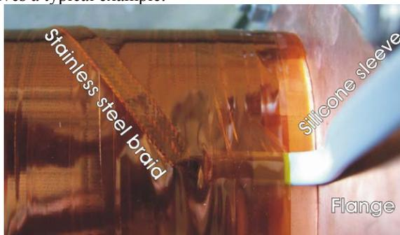
Figure 3: Electrical connection of heater bands.
