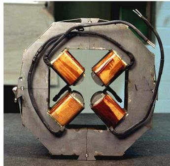
Figure 3: Fermilab 5cm long, 5cm bore quadrupole.
