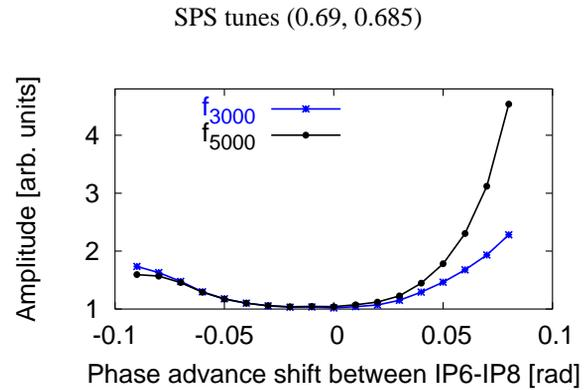
Figure 7: Strengths of two lattice resonances as a function of the horizontal phase advance shift between the two IPs.
