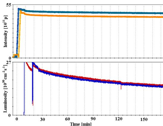
Figure 1: Luminosity decay for a store with 28 bunches. Note that the beam intensity is almost unchanged over the store length.
