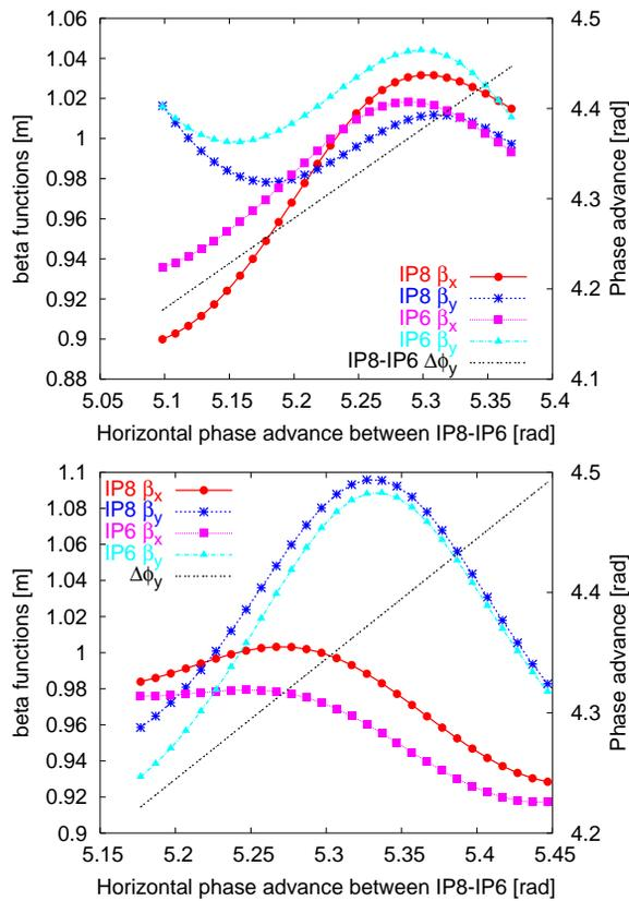
Figure 3: Twiss functions at the IP versus horizontal phase advance for tunes  $(Q_x, Q_y) = (0.225, 0.235)$  (top), and tunes  $(Q_x, Q_y) = (0.69, 0.685)$  (bottom).
