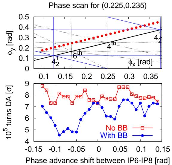
Figure 4: DA for RHIC tunes  $(Q_x, Q_y) = (0.225, 0.235)$ , using all arc quadrupoles to vary the horizontal phase advance between the two IPs (bottom). The top plot shows the working point in the phase advance diagram.
