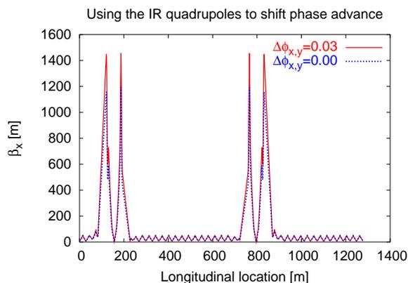
Figure 2: Optics for two phase advance configurations using the IR quadrupoles.
