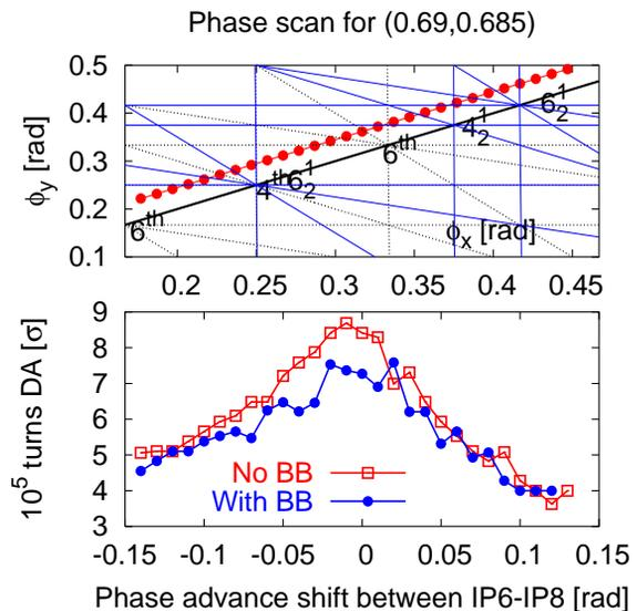
Figure 5: DA for the working point (0.69,0.685) using all arc quadrupoles. The top plot shows the working point in the phase advance diagram.
