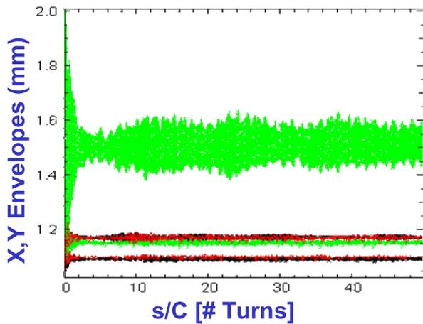
Fig. 3: 2\*rms beam radii for  $\delta=5e-5$  [black], 0.001 [red], and 0.01 [green] velocity spreads, and  $I=0.6$  mA.
