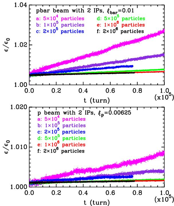
Figure 2: Emittance growth of the  $\bar{p}$  and  $p$  beam due to headon collisions at B0 and D0 calculated with different number of macroparticles in each bunch, where  $\epsilon = \epsilon_x + \epsilon_y$ .
