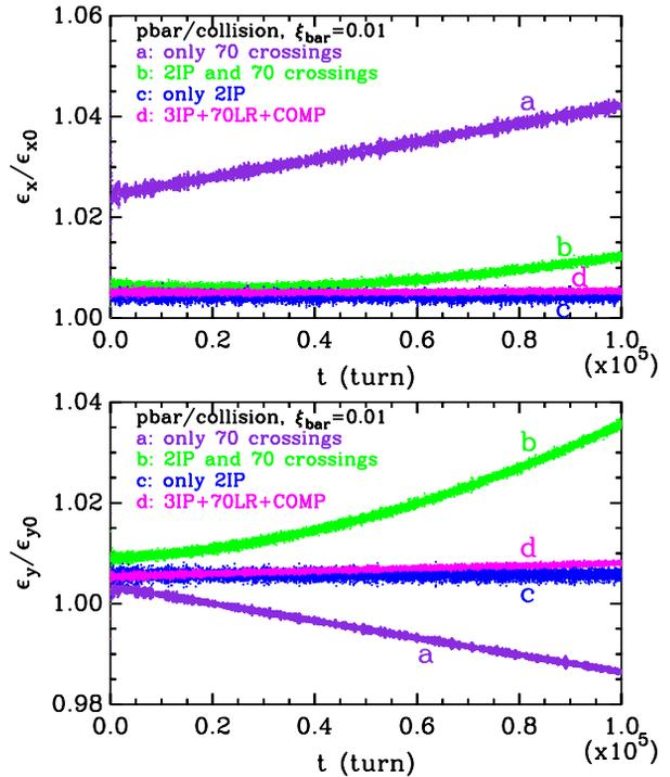
Figure 3: Emittance growth of the  $\bar{p}$  beam in Tevatron during collision with (a) 70 parasitic collisions; (b) 2 headon and 70 parasitic collisions; (c) 2 headon collisions; and (d) the same as (b) but with the multipole compensation.
