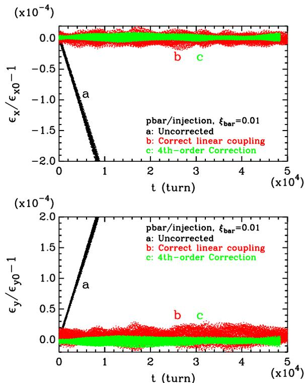
Figure 1: Evolution of the horizontal ( $\epsilon_x$ ) and vertical ( $\epsilon_y$ ) emittance of the  $\bar{p}$  beam at injection energy (a) without any correction; (b) with a correction of linear coupling due to the parasitic collisions and the coupled helix orbit, and (c) with the 3rd-order multipole compensation.  $\epsilon_{x0}$  and  $\epsilon_{y0}$  are the initial emittances
