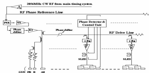
Figure 5: Schematic diagram of the phasing system
