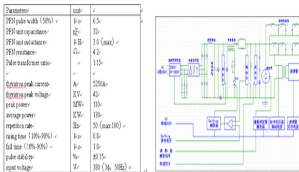
Figure 4: Modulator parameter and the circuit diagram
