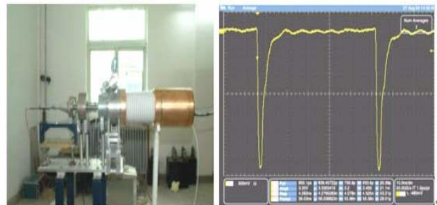
Figure 1: Picture of gun test stand (left) and its produced two pulses(right)
