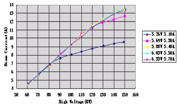
Figure 2: Emitted current vs the gun high voltage
