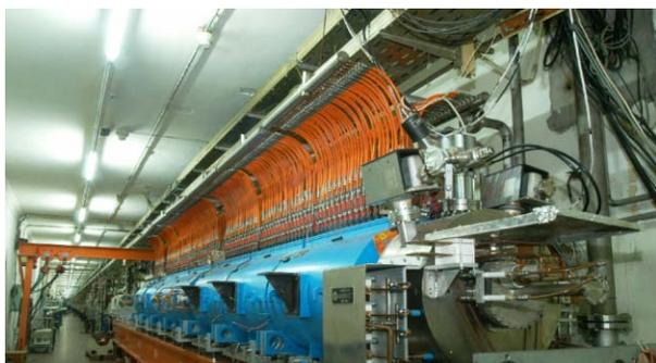
Figure 3: Positron focusing and accelerating system
