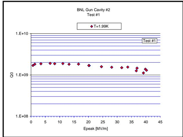
Figure 4, Test Results from Cavity #2 with Aluminum Coupling Probes
