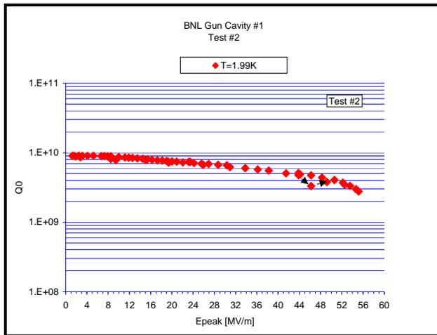
Figure 3, Test Results from Cavity #1 with Nb Coupling Probes.
