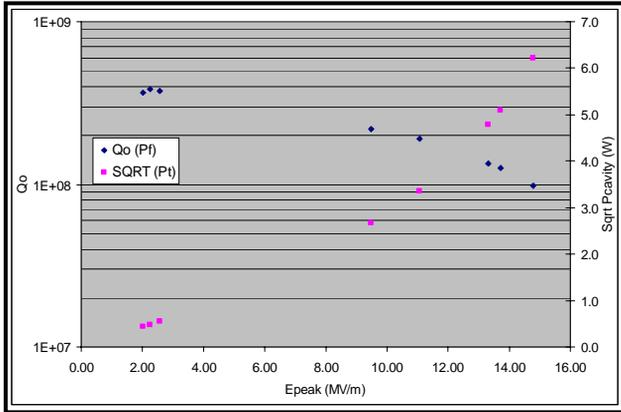
Figure 6, Subsequent 4K Test Results in Operational Cryostat showing  $Q_0$  and the Square Root of the Power Transmitted to the Cavity
