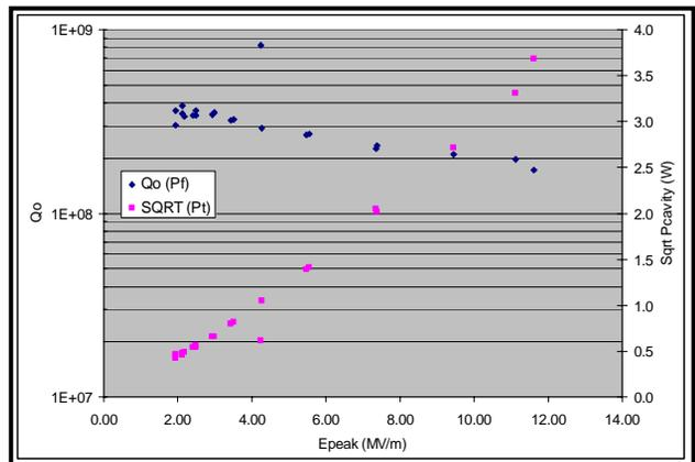
Figure 5, Initial 4K Test Results in Operational Cryostat showing  $Q_0$  and the Square Root of the Power Transmitted to the Cavity
