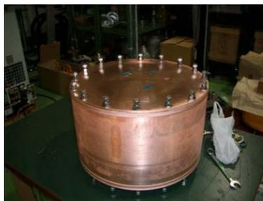
Figure 3: Fabricated pillbox test cavity (after electroplating) used for the  $Q_0$  measurement.
