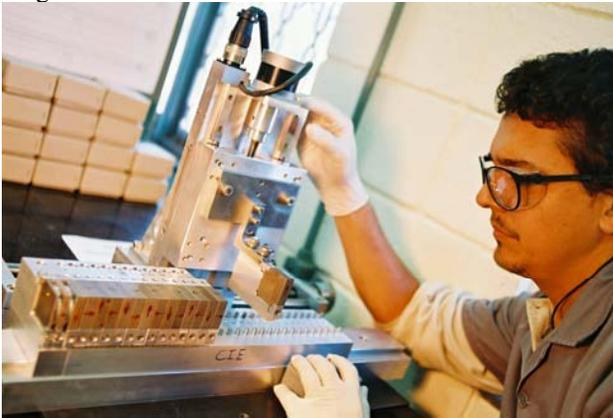
Figure 4: Assembling the prototype Elliptical Undulator.
