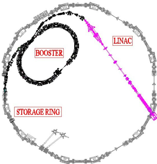
Figure 1: Lay-out of the LNLS Light Source.
