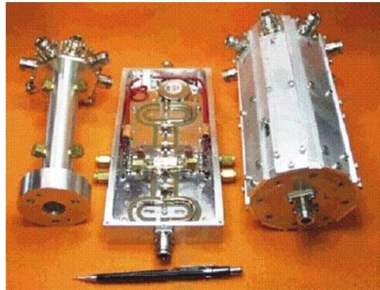
Figure 2: Solid State RF amplifier module and power combiners developed for the booster synchrotron.
