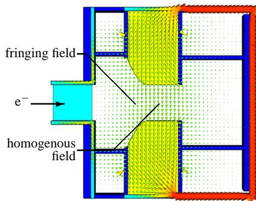
Figure 5: Magnetic Flux Density in the Alpha Magnet
