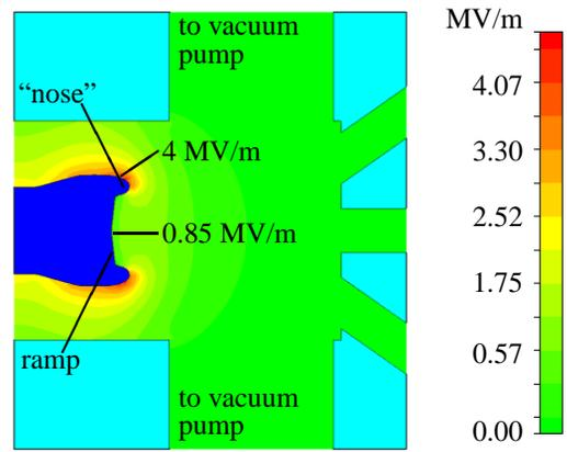
Figure 3:  $|\vec{E}|$  in the source yz plane
