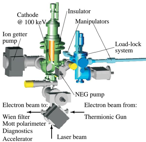
Figure 2: Design of the Injector from Gun to Alpha Magnet
