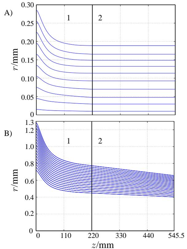
Figure 4: Trajectories of Electron Beam from Photocathode to Alpha Magnet A) by a centered shot and B) by offset shot of 1 mm (1: gun, 2: drift space to alpha magnet)
