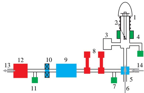
Figure 1: Principal Diagram of the New Low-Energy Injector with 1. Source, 2. Cathode, 3. Load-Lock Chamber, 4. NEG Pump Array, 5. Alpha Magnet, 6. Laser Beam, 7. Differential Pump Stage, 8. Diagnostics, 9. Wien Filter, 10. Solenoid, 11. Turbo Pump Station, 12. Mott Polarimeter, 13. Electron beam to Accelerator and 14. Electron Beam From Thermionic Gun
