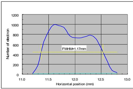
Figure 3a: Horizontally projected beam distribution on the target.
