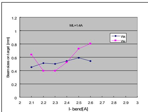
Figure 9b: Beam sizes versus bending magnet magnetic-field strength.
