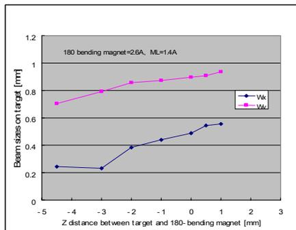
Figure 9d: Beam-sizes measured in the region near the target. The beam is vertically defocused. ( $\theta < 0$ )
