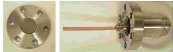
Figure 5b: Be window. Figure 5c: A fixed target.
