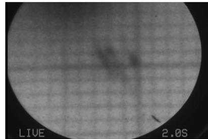
Figure 7a: Picture of a graph paper ruled into 1-millimeter squares observed by a pinhole camera.
