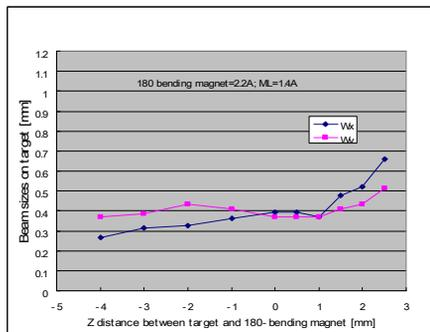
Figure 9c: Beam-sizes measured in the region near the target. Vertical focusing is weak. ( $\theta \sim 0$ )
