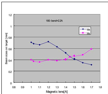
Figure 9a: Beam sizes versus magnetic-field strength.
