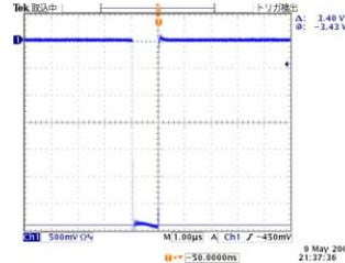
Figure 6: A pulse shape of a  $1\mu\text{s}$  beam operated at 20Hz. The beam current was 68mA as can be reduced from the value on the picture.
