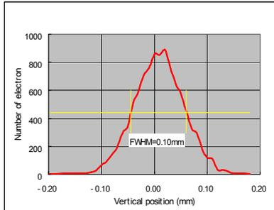
Figure 3b: Vertically projected beam distribution on the target.
