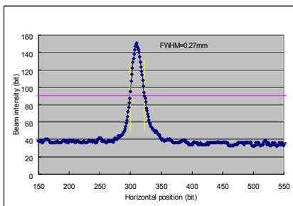
Figure 8a: Horizontal cross section of a beam spot observed by a pinhole camera.
