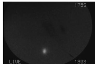
Figure 7b: Typical beam spot observed by a pinhole camera.
