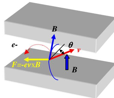
Figure 2: Relation between an injection angle  $\theta$  and a vertical focusing force produced by a fringing field  $B$ .
