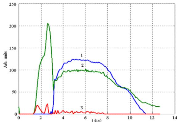
Figure 2: Pulses of voltage (2), beam current (1) and anode current (3), Along the vertical: 1 - 0.4 A/div, 2 - 0.5 kV/div, 3 - 0.04 A/div.
