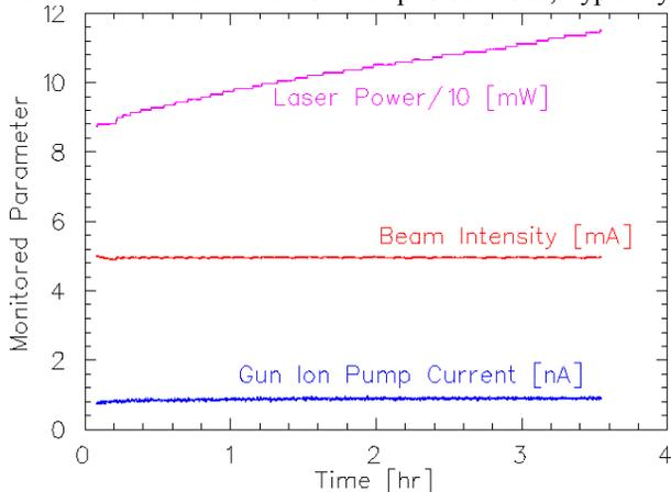
Figure 2: (Color) A 5 mA run; the laser power is automatically increased to maintain constant beam current that, in turn, induces an increased pressure.
