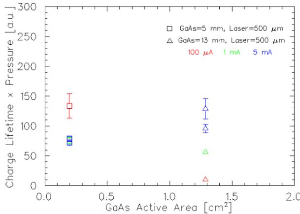
Figure 6: (Color) Product of photocathode lifetime and vacuum pressure versus active area with laser spot size fixed at 500  $\mu\text{m}$ .
