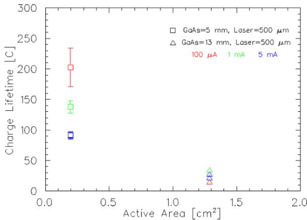
Figure 5: (Color) Photocathode lifetime versus active area with laser spot size fixed at 500  $\mu\text{m}$ .
