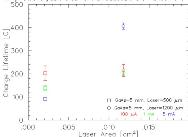
Figure 4: (Color) Photocathode lifetime versus laser spot size with the active area diameter fixed at 5 mm.
