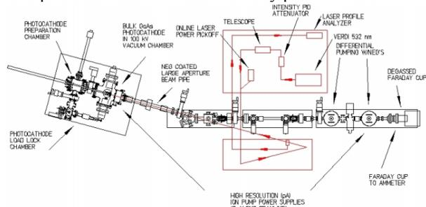
Figure 1: (Color) The 100 kV DC electron gun, beam line and laser system used for this experiment is shown.
