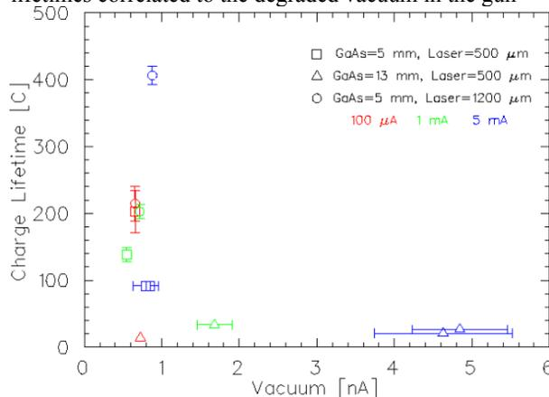
Figure 3: (Color) Photocathode lifetime versus vacuum pressure during the run (base vacuum  $\sim 0.5$  nA).
