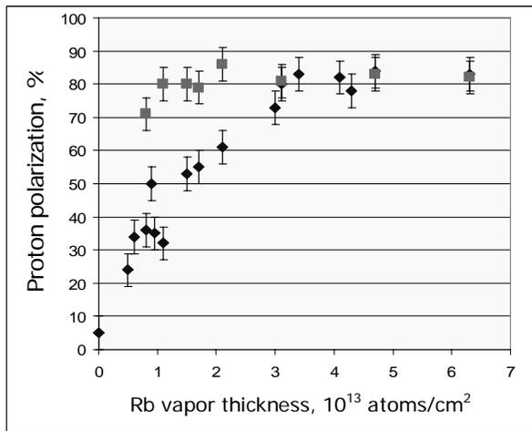
Fig. 2. Proton polarization at 200 MeV vs. Rb vapor thickness before ( $\blacklozenge$ ) and after ( $\blacksquare$ ) the Rb cell upgrade.
