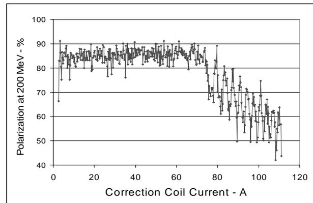
Fig. 4.  $H^-$  Polarization measured at the 200 MeV polarimeter. Sona-shield collimator diameter – 2.0 cm, ionizer solenoid field 1.9 kG.
