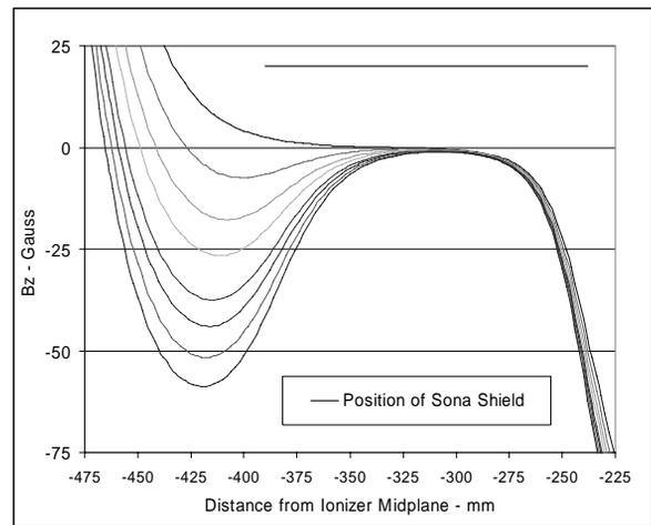
Fig. 3. Calculated magnetic field profiles in the Sona transition region for several correction coil currents corresponding to polarization oscillation peaks.
