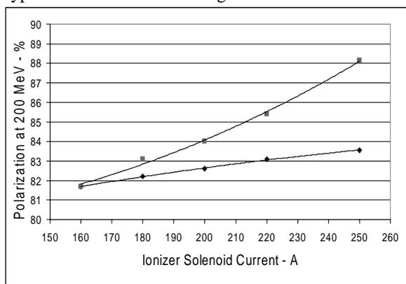
Fig.5. Measured (■) and calculated (◆) polarization vs. ionizer solenoid field strength. Ionizer field at 250 A current is equal to 1.98 kG.
