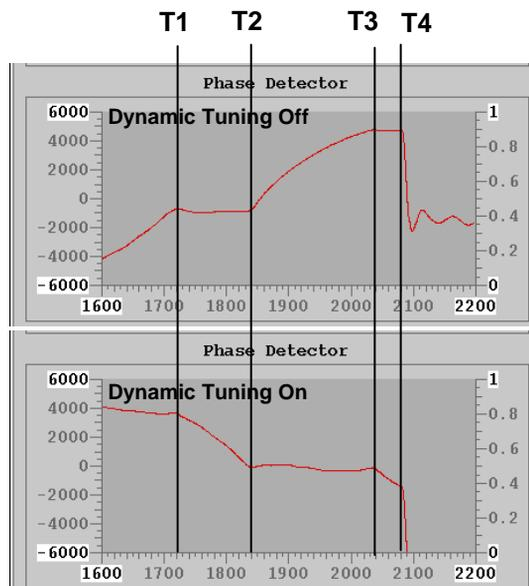
Figure 6: Phase between the grid and anode of the final amplifier stage with and without cavity dynamic tuning.
