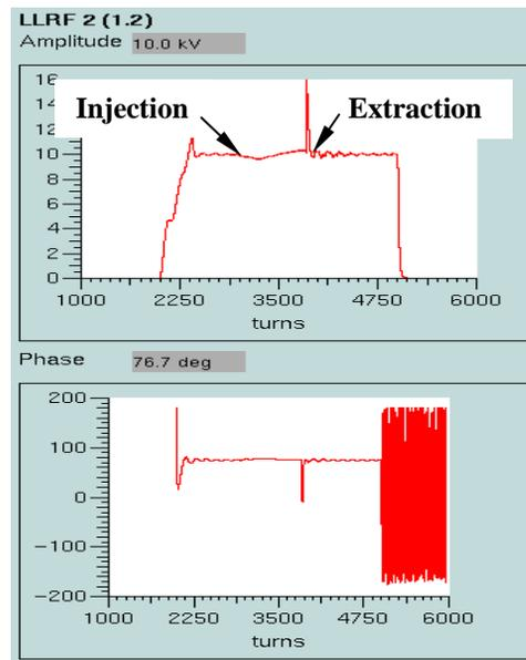
Figure 5: Amplitude and Phase display with  $9.6e13$  protons per pulse.
