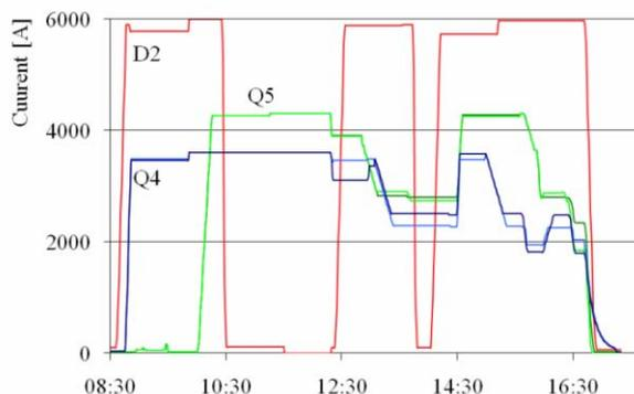
Figure 3: Cycling two apertures of the matching section quadrupoles Q4, Q5 and the separation dipole D2
