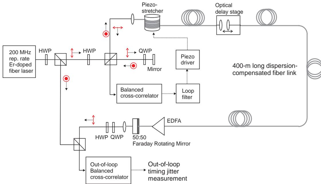
Figure 5: Experimental setup for the fiberlink stabilization.
