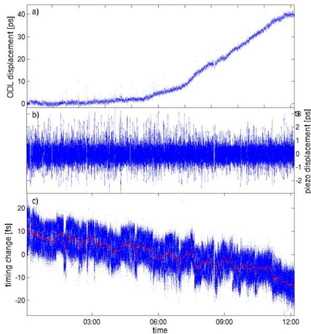
Figure 6: Drift measurement of a 400 m long fiberlink. a) Displacement of the optical delay line (ODL). b) piezo stretcher displacement. c) timing change at the end of the fiber-link. The red line indicates slow timing changes. The timing jitter is  $(4.4 \pm 1.1)$  fs.
