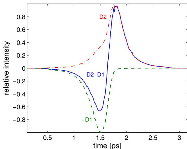
Figure 3: Response of the balanced optical cross-correlator. The signals of the two detectors D1 and D2 (dashed traces) are combined digitally, giving the difference signal (solid trace). Timing jitter measurements are performed at the zero crossing of the difference signal.
