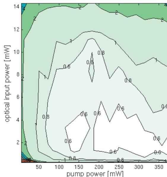
Figure 4: Integrated timing jitter (500 Hz - 4.5 MHz) in femtoseconds added by the EDFA as a function of the optical input power and the power of the 980 nm pump light.
