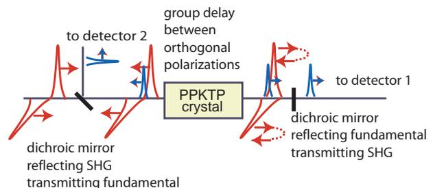
Figure 2: Principle of the balanced optical cross-correlator.
