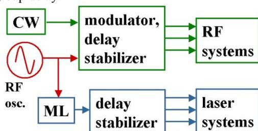
Figure 5: Interconnection of RF and laser sources in Fermi synch system.
