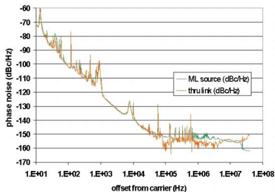
Figure 1: Phase noise of 2.5GHz source and after transmission through AM fiber link.
