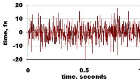
Figure 3: Relative timing jitter of two lasers synched with two-frequency scheme.
