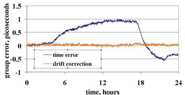
Figure 4: Group delay error of phase stabilized fiber (blue) and calculated with correction factor (orange).
