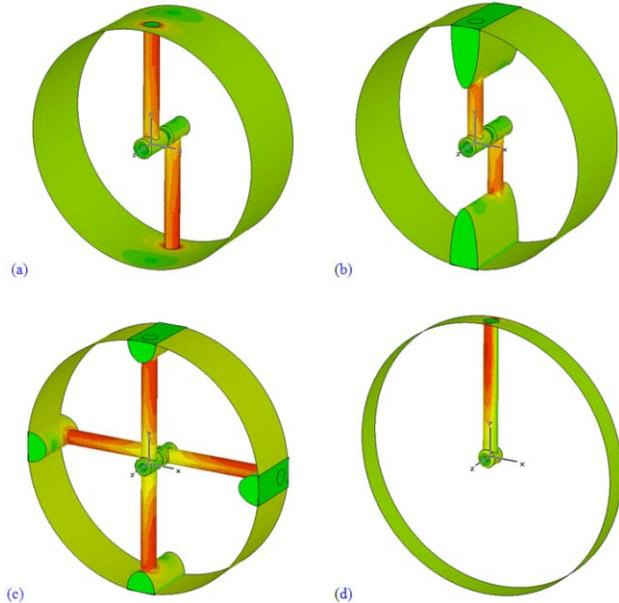
Figure 2: Surface current distributions for the structures in Tab. 3: (a) IH; (b) IH with vanes; (c) CH with small vanes; (d) DTL. See Tab. 3 for spatial and current scales.
