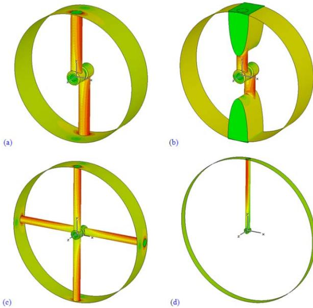
Figure 1: Surface current distributions for the structures in Tab. 2: (a) IH; (b) IH with vanes; (c) CH; and (d) DTL. Red means high current density, green – low. The spatial and current scales are different in all pictures, cf. Tab. 2.
