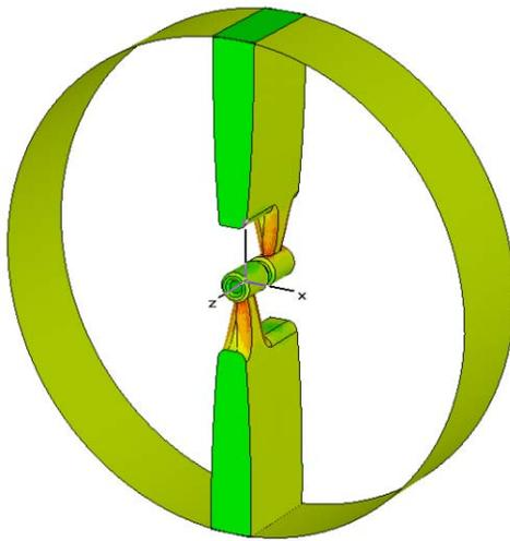
Figure 3: Surface current distribution for the modified IH structure with vanes at  $\beta = 0.034$ , with  $Z_{sh}T^2 = 746 \text{ M}\Omega/\text{m}$ .
