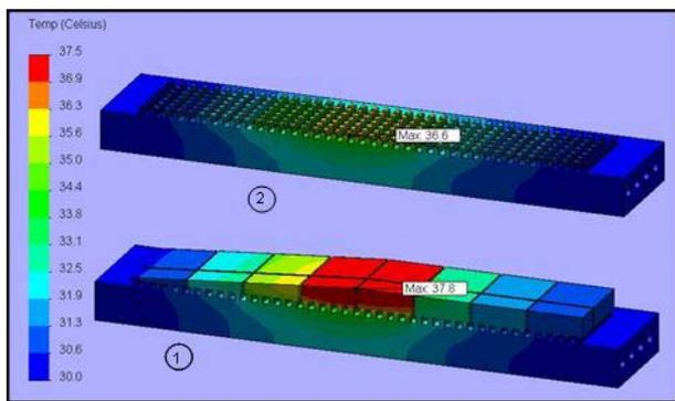
Figure 6: Temperature distribution in the dampers. 1-Entire structure; 2-copper substrate.
