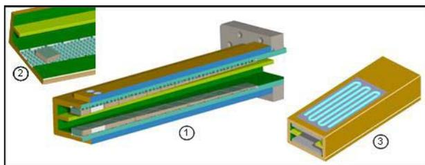
Figure 5: Damper structure. 1-Section view of the structure; 2-individual SiC tile brazed atop the copper pin matrix; 3-cooling channels incorporated in copper walls.
