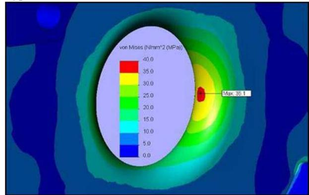
Figure 4: Thermal stresses calculated for 15-mm-thick iris of a ‘typical’ cell.
