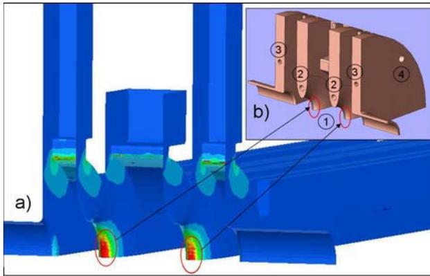
Figure 2: Power deposition at the surfaces of normal-conducting deflecting cavity at APS. a) HFSS computations, b) solid model of the cavity proper (no waveguides). 1-Regions of peak power generation; 2-cooling channels in coupler cell irises; 3-cooling channels in end cell irises; 4-peripheral cooling (optional).
