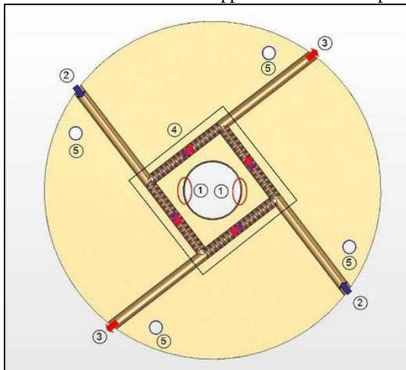
Figure 3: Schematics of the cavity cooling. 1-Regions of peak power generation; 2-water inlets; 3-water outlets; 4-the region of intensified convective cooling; 5-peripheral cooling (optional).
