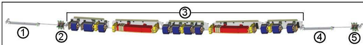
Figure 1: Layout of Short X-Ray Pulse System at the APS. 1-Sector 6ID Undulator vacuum chamber; 2-the first pair of the cavities; 3-sector 7ID girders; 4-sector 7ID undulator vacuum chamber; 5-the second pair of the cavities.
