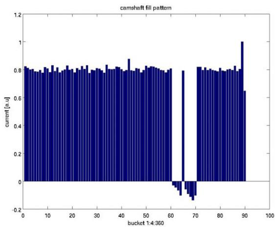
Figure 3: A successfully injected "camshaft" fill pattern.
