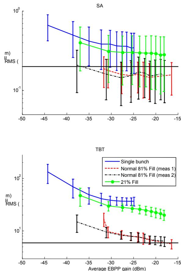
Figure 1: Average resolution of 96 BPMS for SA data (top) and TBT data (bottom). The error bars are a one sigma spread of the resolutions across 96 BPMS. The solid horizontal lines are the values in the specifications. "81% fill" means a continuous fill of 81% of the buckets in the storage ring. Single bunch measurements were taken in 1 mA steps from 1–10 mA. 21% fill measurements were taken in 3 mA steps from 3–30 mA. 81% fill measurements were taken in 10 mA steps from 10–100/125 mA.
