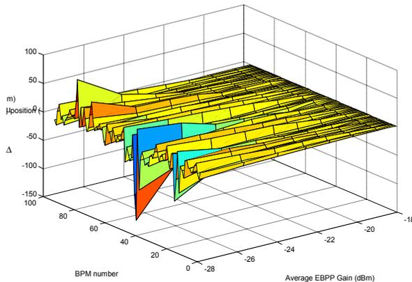
Figure 2: The plot above shows the absolute change in the beam position with respect to the beam position at 100 mA (gain  $\sim -18$ ) for all the BPMs in the storage ring.
