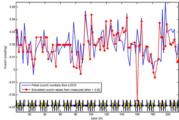
Figure 3: A good correlation between simulated crunch values based on measured attenuations and calculated values using LOCO. The 2% offset in the simulated data reflects the inherent coupling on the EBPP's analogue board.
