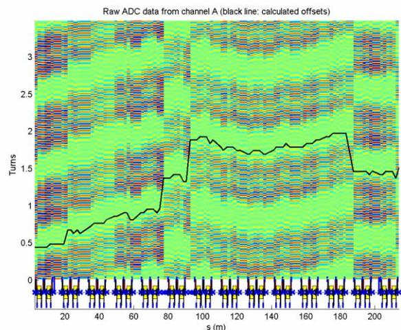
Figure 4: The above is a surface plot of raw data directly from the ADC on one channel of the EBPPs. The vertical axis is time measured in units of the revolution period and shows that for a given turn, the synchronicity between BPMs is out by  $\sim 1.5$  turns (1.08  $\mu\text{s}$ ). The solid line represents the calculated delay given by the time of flight and various signal delays.
