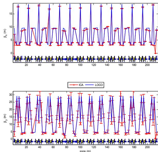
Figure 5: Plot of horizontal (top) and vertical (bottom) beta functions at the BPMs as calculated using ICA and LOCO. Error bars in the ICA calculated betas represents a one sigma spread from the 4 data sets. The beta beating seen in the ICA plot is not reflected in the LOCO plot.
