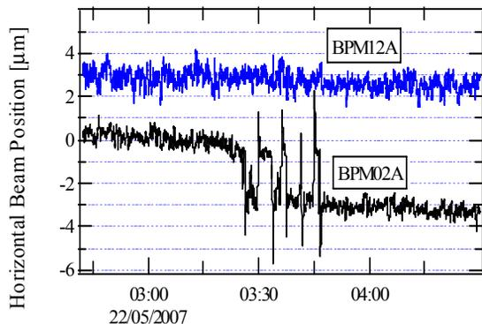
Figure 1: False BPM reading with daily regularity that appears always in the same stripline BPM when the beam current reaches a specific value. So far we have observed three BPMs with this behavior. The current in which the problem occurs is different for each BPM.
