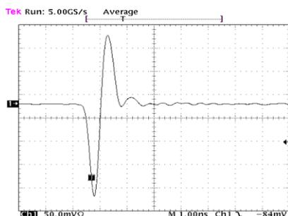
Figure 5: Button signal with a 2.5 mA single-bunch in the storage ring. The signal symmetry and the amplitude of the reflections indicate that the impedance matching provided by the cone above the button is efficient.
