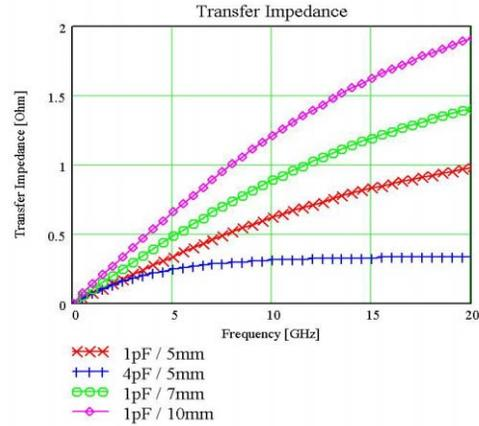
Figure 3: Modulus of the transfer impedance calculated for some values of button capacitance and button radius. In the low frequency region the button capacitance does not affect the transfer impedance, but a small increase in the radius impacts significantly the transfer impedance value.
