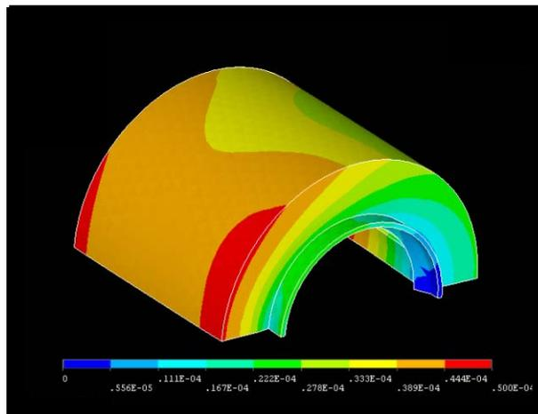
Figure 2: Numerical simulation showing mechanical deformations on the BPM caused by temperature differences along the 316L stainless steel BPM body. Temperatures as high as 300 °C in the BPM areas near the beam plane can cause 100-μm asymmetries in the striplines. Note that the striplines are free in one extremity making the heat exchange more difficult in this region.
