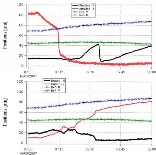
Figure 6: External heating experiment with a stripline and a button BPM. In both graphs there are reference readings from one BPM that had not been heated.
