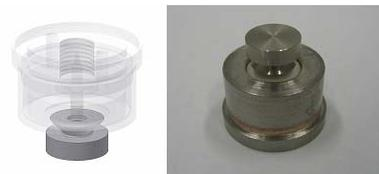
Figure 4: Button mechanical design and button after complete mounting (before soldering in the BPM body). The cone above the button creates a 50  $\Omega$  tapered transmission line with the BPM wall.
