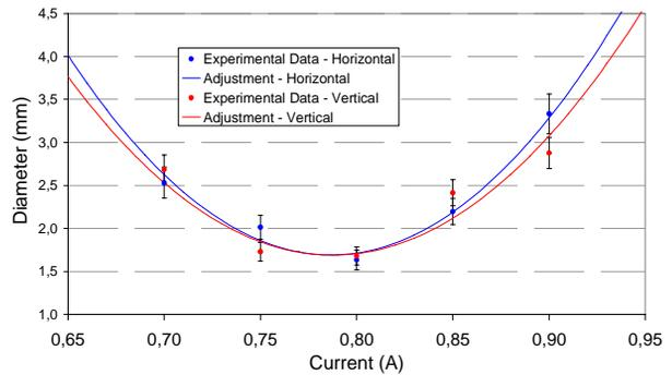
Figure 3 – Beam diameter as function of the excitation current in the second lens.
