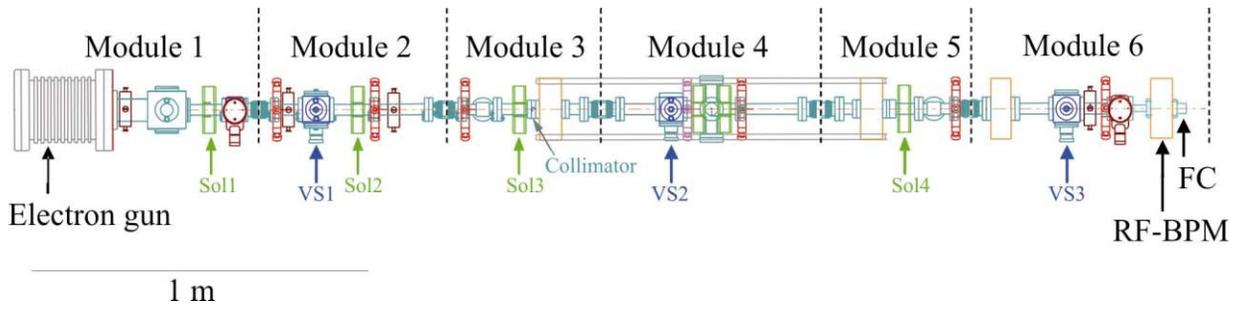
Figure 2 - The conforming stage of the injector linac of the IFUSP microtron: FC stands for Faraday Cup, and RF-BPM for radio frequency beam position monitor.
