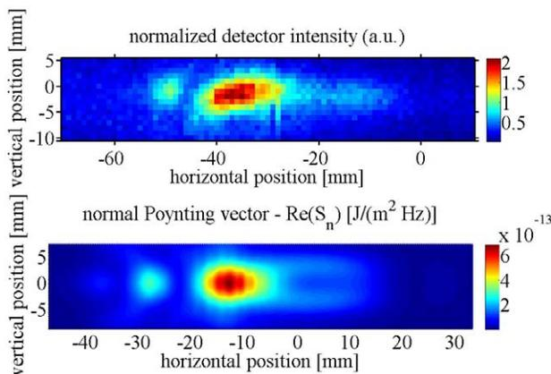
Figure 3: Comparison of measurement (top) and simulation (bottom) at  $\lambda = 155\mu\text{m}$ .
