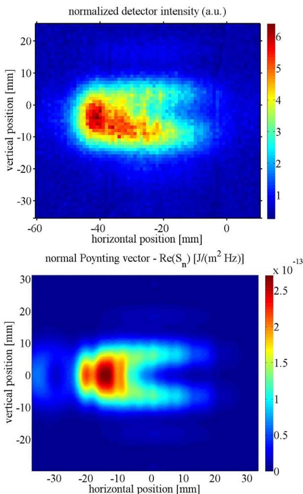
Figure 2: Comparison of measurement (top) and simulation (bottom) for the synchrotron radiation intensity at a distance of 220mm in front of the waveguide exit as seen from inside the vacuum chamber at  $\lambda = 350\mu\text{m}$ .
