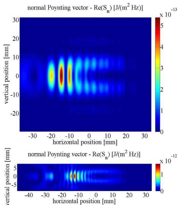
Figure 4: Unfiltered simulation results for the reference frequencies  $\lambda = 350\mu\text{m}$  (top) and  $155\mu\text{m}$  (bottom).
