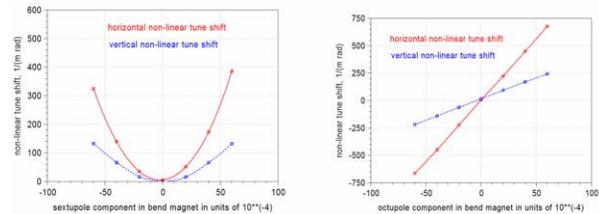
Figure 3: The non-linear tune shift vs. the sextupole  $\Delta b_{sext\_mag} / B_0$  and octupole  $\Delta b_{oct\_mag} / B_0$  components in bend magnet.
