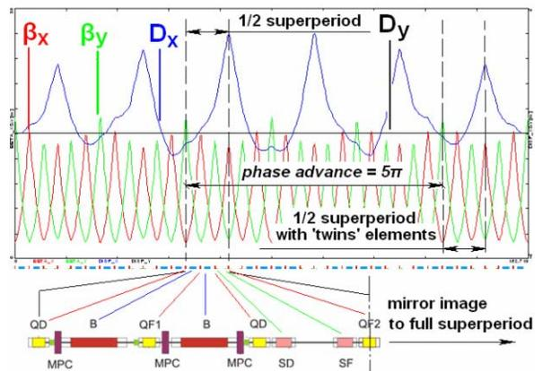
Figure 2:  $\beta$ -functions and dispersion on the arc (6-fold symmetry option).
