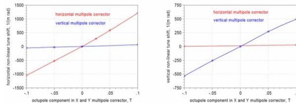
Figure 4: The non-linear tune shift versus the octupole components in multipole horizontal  $b_{oct}^{hcor}$  and vertical  $b_{oct}^{vcor}$  correctors.
