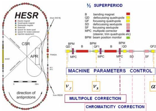
Figure 1: Schematic layout of the HESR lattice with the half superperiod of arc.
