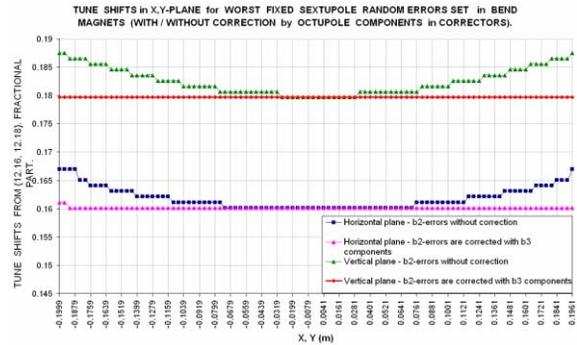
Figure 6: Tune shifts (from sextupole errors) vs. particles amplitude with / without octupole correction.
