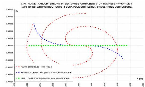
Figure 7: The phase space filamentation due to random sextupole errors in the bend magnets and the multipole correction scheme.
