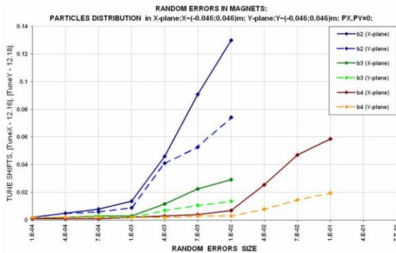
Figure 5: Betatron tune shifts vs. the random errors size ( $|\text{tune}_{x,y} - (12.16; 12.18)|$ ).
