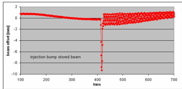
Figure 13: Orbit bump induced by the Septum and the Kickers in the injection section.
