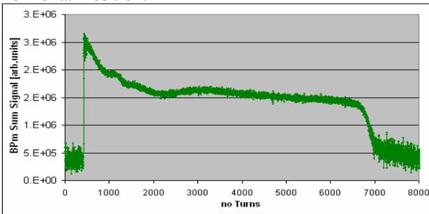
Figure 6: Sum Signal from the injected beam without RF.
