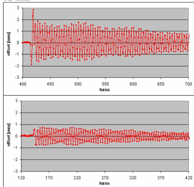
Figure 14: Orbit oscillation due to the kickers before and after optimization.
