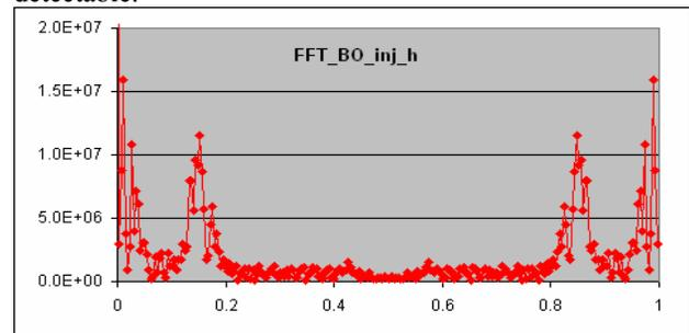
Figure 2: FFT of the horizontal Booster orbit at Injection.
