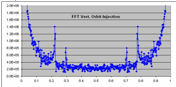
Figure 12: FFT of the vertical SR orbit at injection with 100 mA accumulated, excited by the injection.
