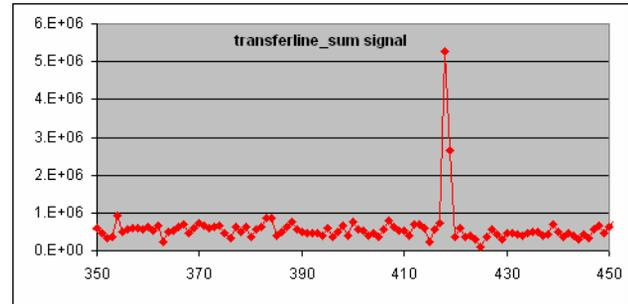
Figure 1: Sum signal from a BPM in the Booster to Storage ring transfer line. The bunch train is 70 ns long. The turn by turn spreads it over 2 turns (736 ns).
