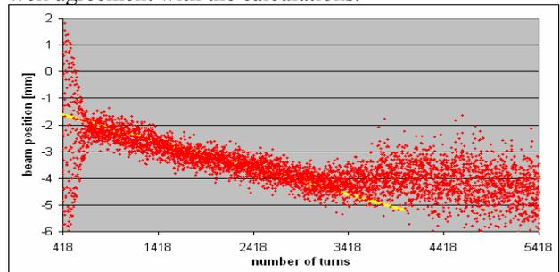
Figure 10: Horizontal Orbit for a BPM with dispersion. The yellow line shows the expected orbit drift due to the energy loss given by the Synchrotron Radiation.
