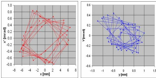
Figure 11: Horizontal and vertical Phase space for the injected beam calculated from two BPMs.
