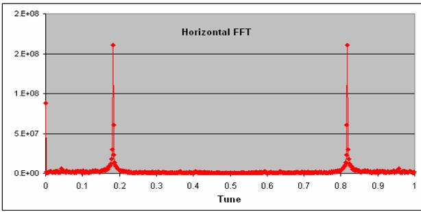
Figure 4: FFT of the horizontal orbit after excitation by the extraction kicker.
