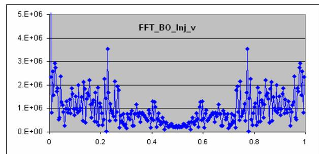
Figure 3: FFT of the vertical Booster orbit at Injection.
