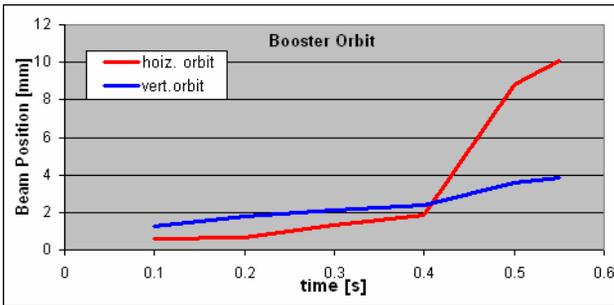
Figure 5: Horizontal and vertical orbit in the booster. The large jump after 0.4 s is due to the excitation of the bumper magnets for the extraction.
