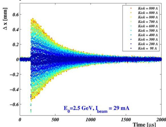
Figure 1: Time evolution of the horizontal centre-of-charge position averaged over all 32 bunches of a train after an excitation with a kicker magnet. The different datasets represents measurements with different kicker strengths. The measurements were performed at a beam energy of 2.5 GeV with a total beam current of 29 mA.
