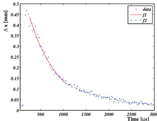
Figure 6: Envelope of the measurement shown in Fig. 6. The red and green curves are to exponential fits to separate regions of the data. The exponential describing the second part of the dataset exhibits a damping time of about 1.2 ms and twice as long as the damping time of the first part exponential (640 μs).
