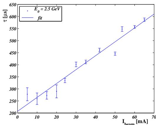
Figure 8: Damping times of the second part extracted from the measurements with different beam currents in Fig. 7 as a function of the beam current.
