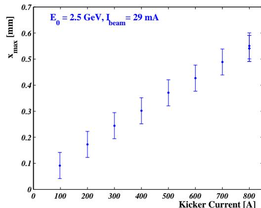
Figure 2: Start amplitude, measured after the decay of the exciting kicker pulse, as a function of the kicker current for the datasets displayed in Fig. 1.
