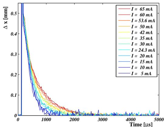
Figure 7: Envelopes of the multi-turn datasets taken at 2.5 GeV for different total beam current in the 32 bunches of one train. After an initial time where all datasets show a comparable behaviour, the damping time decreases with the beam current.
