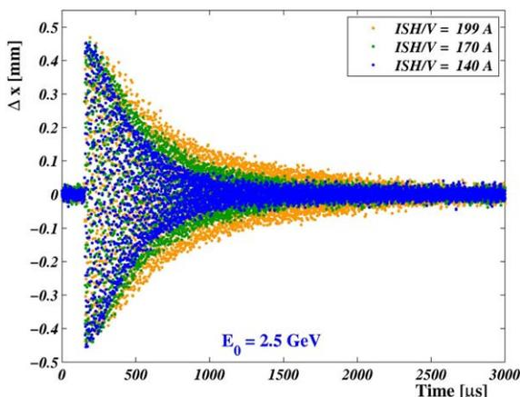
Figure 4: Centre-of-charge position after a kick measured at a beam energy of 2.5 GeV for different currents of the horizontal and vertical sextupoles. For each dataset, the sextupoles currents are approximately equal.
