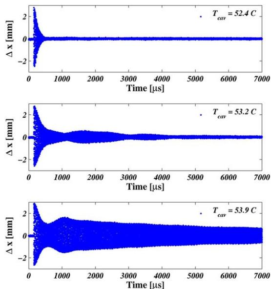
Figure 9: Time evolution of the centre-of-charge measured at a beam energy of 1.3 GeV with a beam current of 10 mA. The three plots show datasets for different cavity temperatures, that is different states of longitudinal excitation. The dataset for the highest temperature, 53.9°C, was longitudinally completely stable whereas a longitudinal instability was excited for a temperature of 52.4°C.
