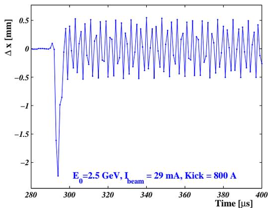
Figure 3: Centre-of-charge position for the first turns after the excitation. The kicker’s pulse length of about 3 μs is clearly visible in the data.
