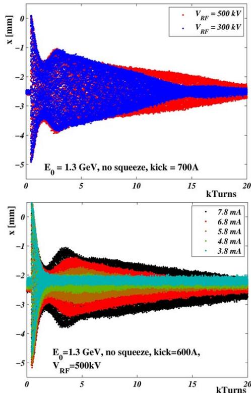
Figure 10: Centre-of-charge evolution at a beam energy of 1.3 GeV in a longitudinally stable state for two different RF voltages. (top) and for different total beam current (bottom). The rise time of the instability is clearly a function of current as is the effective damping time. A higher voltage leads to a longer effective damping than a lower voltage.
