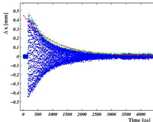
Figure 5: Multi-turn dataset (blue) with the corresponding envelope (green). The red curve is an exponential fit to the measurements. Obviously a simple exponential is not sufficient to describe the dataset.
