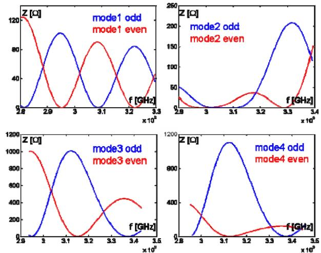
Figure 4: Coupling impedance of the 8 TE<sub>11</sub>-like trapped modes as a function of their frequency.
