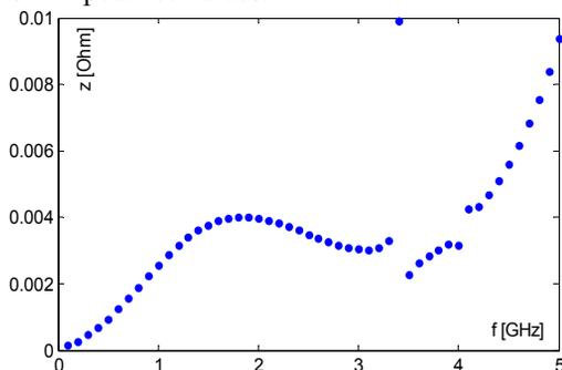
Figure 7: Shielded bellows coupling impedance.
