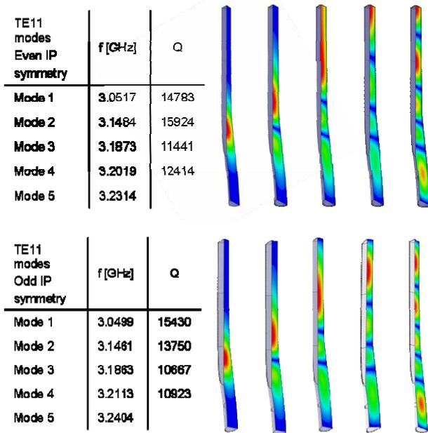
Figure 2: List of the first 10 TE<sub>11</sub>-like modes found by HFSS eigenvalue solution with even and odd symmetry conditions with respect to the IP. The 5<sup>th</sup> mode frequency is above the cut off of the pipe.
