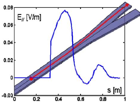
Figure 3: Electric field component tangential to the beam trajectory for the mode2 odd (from HFSS simulations).
