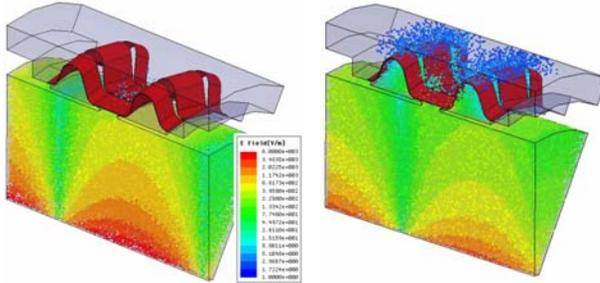
Figure 6: Beam generated fields in the shielded bellows at 3 GHz (HFSS simulations). Left: strips in contact with the cylindrical shells. Right: 0.3mm gap between them.
