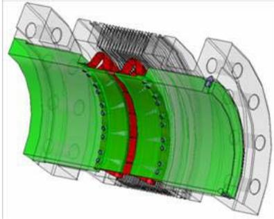
Figure 5: The new IR shielded bellows (a quarter section).
