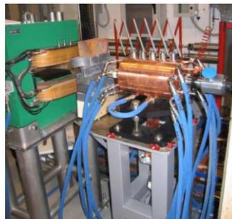
Figure 6: RF deflector installed in SPARC.
