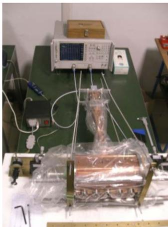
Figure 4: Measurement setup with the device before brazing.
