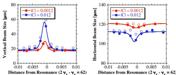
Figure 3: Vertical (left) and horizontal (right) beam sizes in the vicinity of the skew sextupole resonance.
