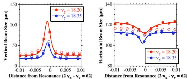
Figure 4: Vertical (left) and horizontal (right) beam sizes in the vicinity of the skew sextupole resonance with different distances from the linear difference resonance.
