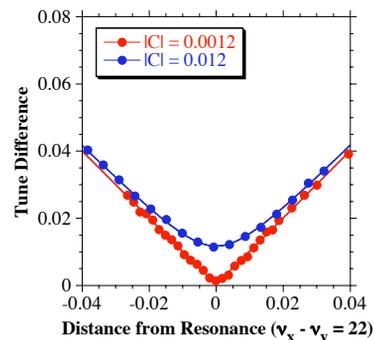
Figure 1: Tune difference in the vicinity of the linear coupling resonance.
