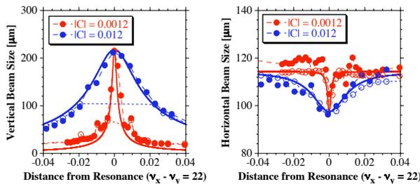
Figure 2: Vertical (left) and horizontal (right) beam sizes in the vicinity of the linear coupling resonance.
