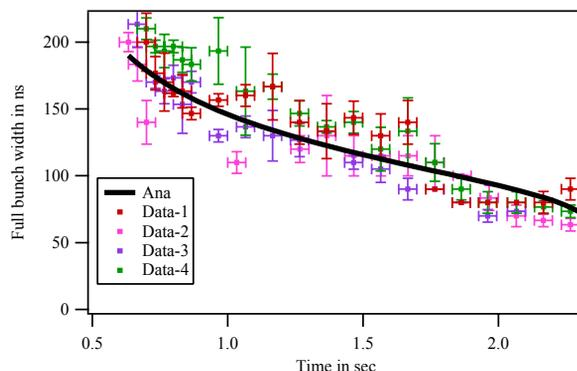
Figure 3: Comparison between the experimental results and theoretical predictions after 0.633 sec from injection.
