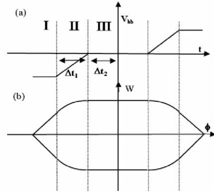
Figure 2: (a) Barrier voltage profile with three distinct regions and peak height of  $V_0$ . (b) Typical trajectory in the phase space.
