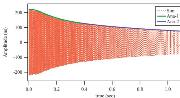
Figure 4: Comparison between the simulation results and theoretical predictions for ideal trapezoidal barrier.
